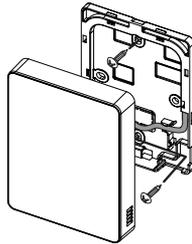
※ You must fit the screws into the screw holes.
