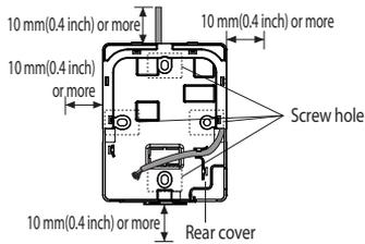
※ Before fixing the rear cover, secure at least 10 mm (0.4 inch) space of upper side, left side, right side, and bottom side.
