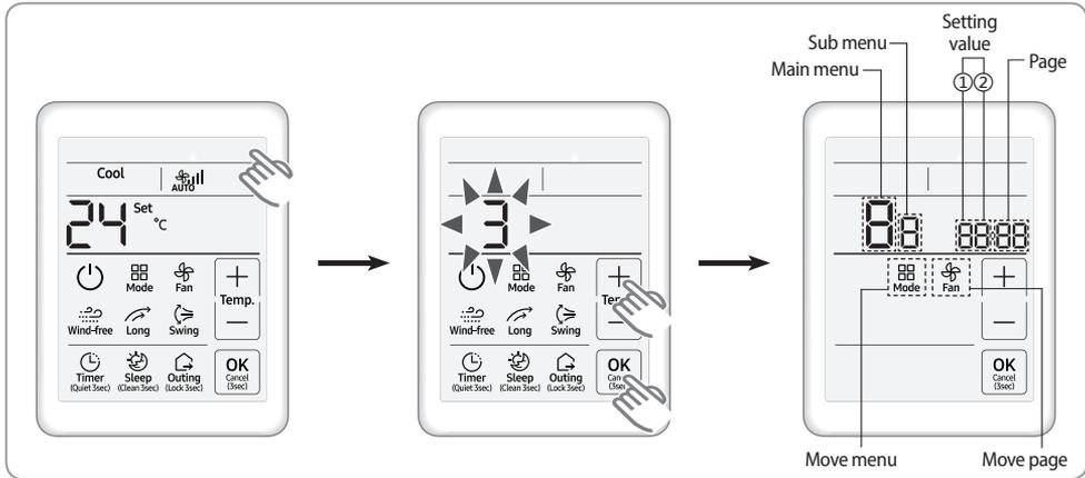
1. If you want to use the various additional functions for your wired remote controller, press the top right corner (hidden button) of the display for more than 3 seconds and drop it. Then you can press [ + ]/[ - ] buttons and select No.3 and press [ **OK** ] button.
