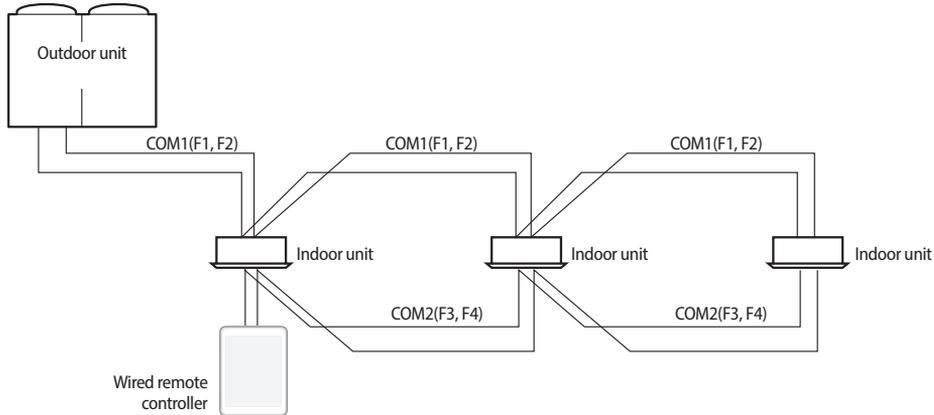
2. Using one wired remote controller to control indoor units connected to different outdoor unit
