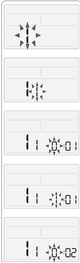
1. Press the top right corner (hidden button) of the display for more than 3 seconds and drop it. Then you can press [ + ]/[ - ] buttons and select No.3 and press [ **OK** ] button.
