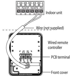
※ Do not tighten the screws on the PCB terminal with excessive force.
